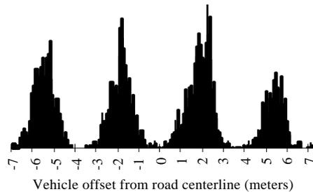
**Fig. 1. Distribution of GPS based vehicle positions across roadway.**
