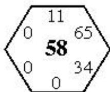
**Fig. 5. Cell of a map representation suitable for lane departure warning. The central element is the probability of a car on the segment passing through the cell. The peripheral numbers are the probability that a car leaves by the nearby face of the hexagon.**
