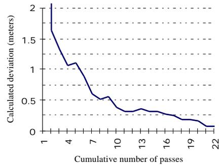
**Fig. 3. Reduction in the calculated deviation of the map from the ideal centerline as the number of vehicle passes increases.**
