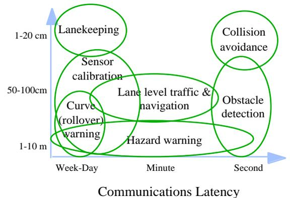
**Fig. 4. Example applications as a function of position accuracy and communications latency**
